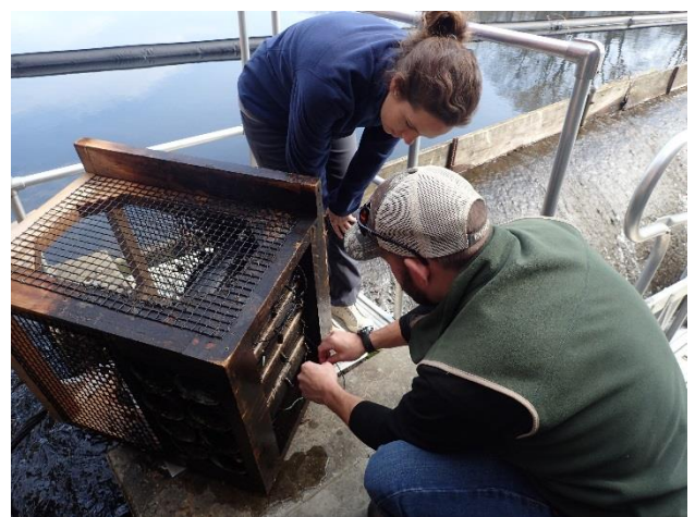
Amanda Ryan (Town of Greenwich) and Dave Ellis (DEEP) reattach a loose wire for the fish counter at the Mianus Pond Fishway. The box-like object slides down into the fishway exit and fish swim through it to be counted.
